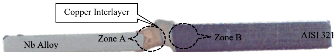
Figure 3: Optical cross sectional micrograph of weld specimen.
