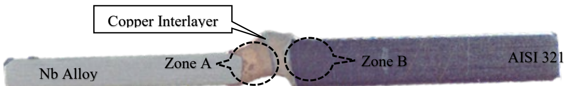
Figure 7: Optical cross sectional micrograph of weld specimen.
