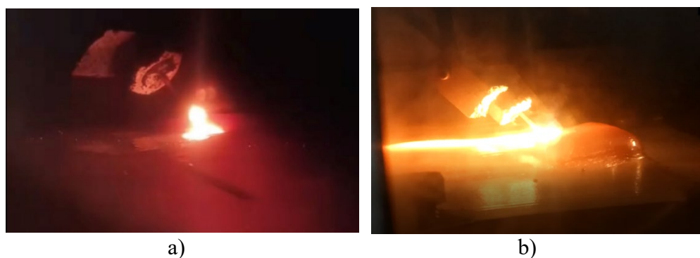
Figure 3 – ELAT Sample Formation Process: a) the first layer; b) fifth layer
